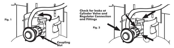
5. Check for leaks by brushing the soap solution on all gas valves, hose connections and fittings. (Shown by the heavy arrows in Fig. 2 & 3) Make sure you generously brush the locations with the soap solution, completely surrounding the connections and fittings.
